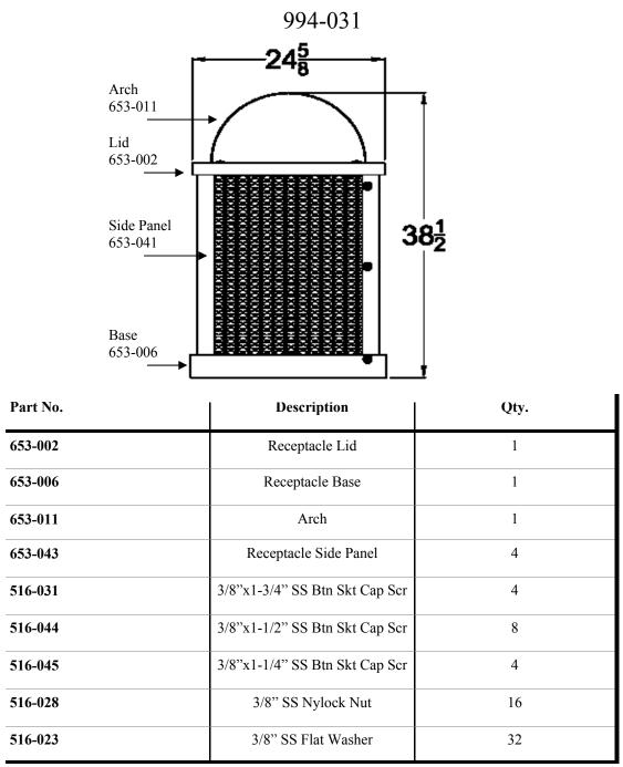
1. With a 7/16" drill bit, drill out the holes of the side panels, arch, lid, and base.
